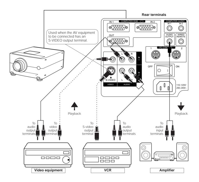
Select the audio you want to output by selecting VIDEO 1 or VIDEO 2. Note the following when using the S-VIDEO INPUT terminal:
